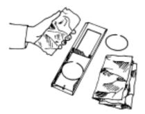
Fig. 1—Typical mounting for flexible fabric specimens.
