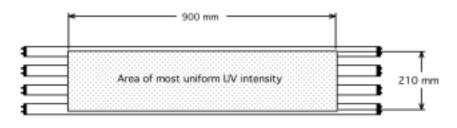
Fig. 4—Area of most uniform light intensity.
