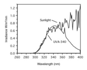
Fig. 3—Representative spectral power distribution, UVA-340 fluorescent lamps
